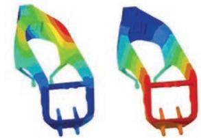
**TOP:** The multibody model built in Altair MotionSolve and Altair HyperWorks enabled the team to determine the occurring dynamic loads. **MIDDLE:** Aerodynamic simulation of the model in a virtual wind tunnel to assess the aerodynamic forces on the bracket. **BOTTOM:** Using the Altair solutions, a mass reduction of 30% was achieved while maintaining the stiffness of the original part.
