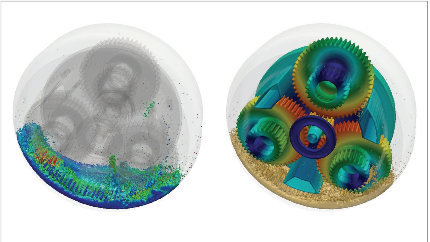
nanoFluidX is a particle-based (SPH) fluid dynamics simulation tool to predict the flow in complex geometries with complex motion. It can be used to predict the oiling in powertrain systems with rotating shafts / gears and analyze forces and torques on individual components of the system. Utilizing the GPU technology empowers high-performance simulations of real geometries.
